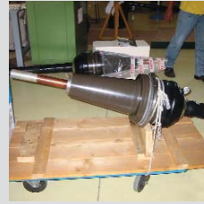
TERMINATION READY FOR FINAL POSITIONING
