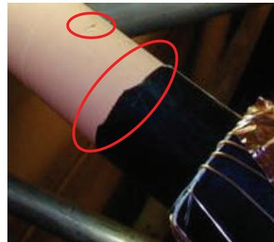
Poor cutbacks and insulation nicks, such as shown here, can result in a corona discharge and premature cable failure. So, why take the chance with splices when, in many cases the
