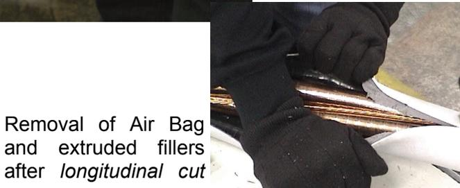
Removal of Air Bag and extruded fillers after longitudinal cut
