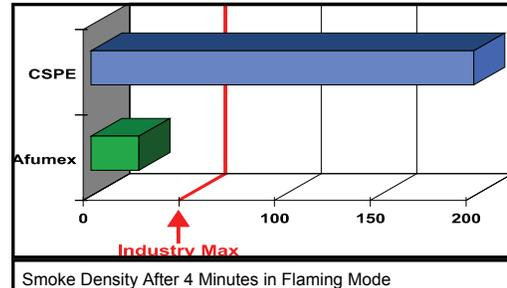
generation be eliminated. The industry standard measurement in this regard is the NBS Smoke Chamber test. Prysmian's EcoSafe™ design emits approximately 50% less smoke than the industry recognized 'low smoke' requirement. This easily earns an 'LS' rating in accordance with UL 1685 as well as a 'low smoke' qualification in accordance with ICEA T-33-655.
