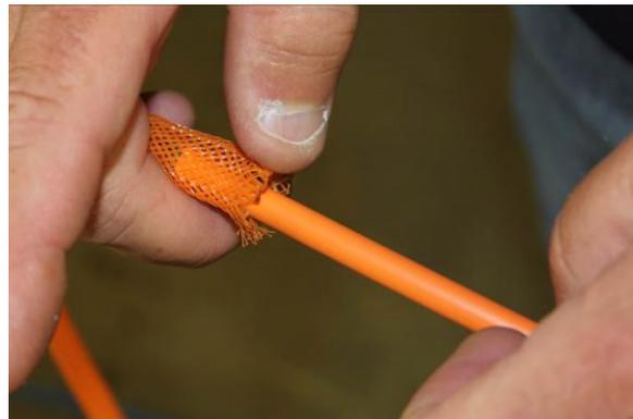
The pictured material is Techflex Flexo PET 3/8" ([www.techflex.com](http://www.techflex.com)). Other materials can be used, provided they don't put excessive pressure on the fibers, or kink when stored.
