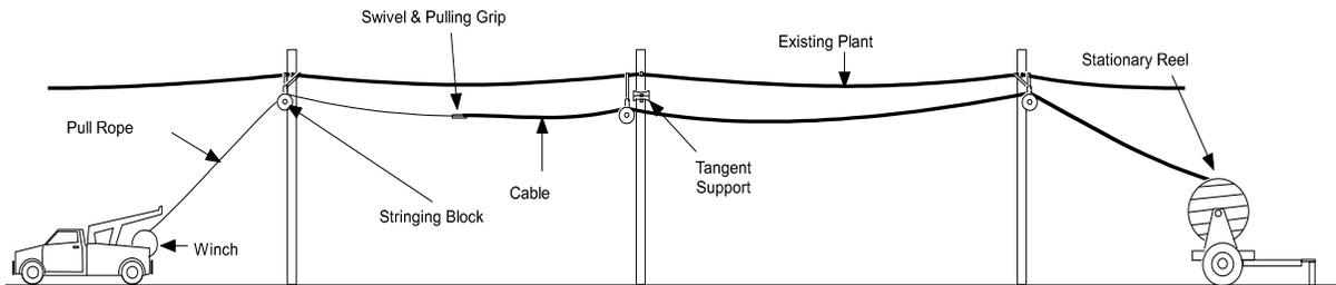
Figure 1 - Stationary Reel Method of Cable Deployment
