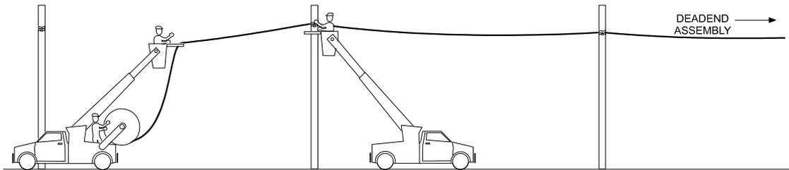
**Figure 4 - Drive Off Method of Cable Deployment**
