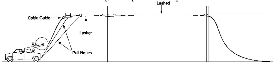
Figure 1. - The Moving Reel Method of Cable Placement
