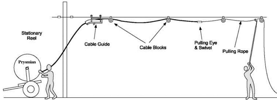
Figure 8 - Setup for Stationary Reel Method
