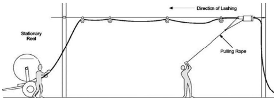
Figure 10 - Pull-back Lashing of Cable
