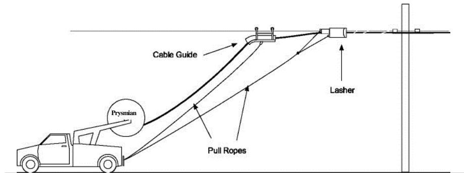
Figure 7 - Setup for Moving Reel Method
