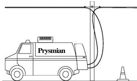
from strand level to a splicing vehicle below plus 16 feet or so of extra slack.
