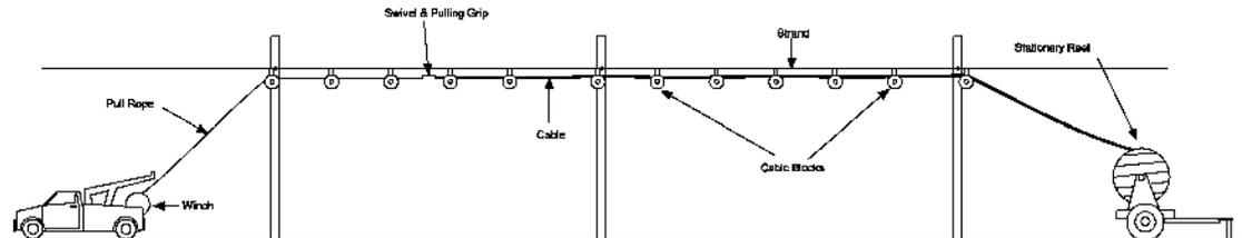
Figure 2. - The Stationary Reel Method of Cable Placement
