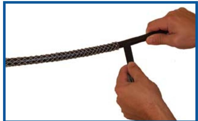
10. Connect the pulling eye to an approved breakaway and swivel. The grip installation is complete, and the cable is ready to be pulled.
