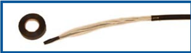
Note: For central tube designs, it is recommended that two additional wraps of vinyl tape be applied around the base of the ring cut to prevent the strength members from catching the mesh of the grip during installation.
