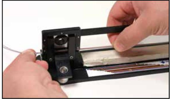
**1.8** Allow glue to dry and remove fiber from holder. While holding the ribbon, unhook the bracket(s) and slowly lift up the ribbon.
