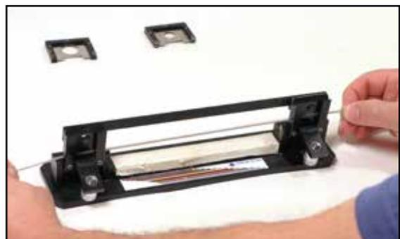
**1.6** While maintaining gentle pressure on the fiber ends tighten the fiber clamps.
