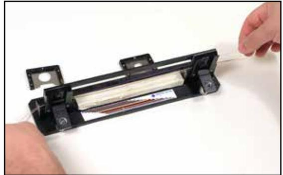
**1.4** Place the fiber ends so they extend 2 to 3 inches beyond the tool. Insert the holding clips into position to hold the fibers in place.
