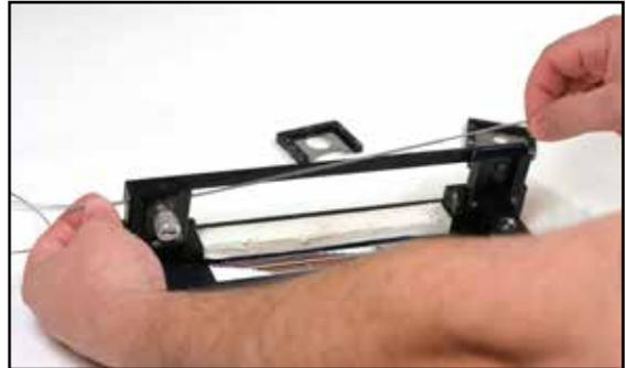
**1.9** Snip the excess fiber ends that are not ribbonized in preparation for splicing.
