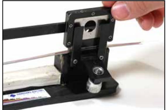
**1.5** Grasp the fibers and pull them back, aligning the fiber ends within a 1/2-inch of the tool's edge.
