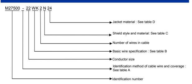
Table A: Identification method of Cable Wire (with Shield Coverage)
